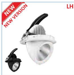
HLR-2425 (40W / 50W) Size : Ø190mmx158mm Cut-Out : Ø175mm Body Colour Available : White / Black
