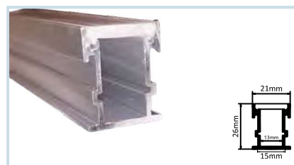
HLL-1078 : CONCELED BODY FULL SET STANDARD LENGTH : 3MTR SIZE : 21mmxD26mm / CUT-OUT : 15xD23mm
